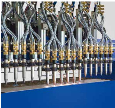
The machine can be equipped with a maximum of 20 oxyfuel torches
